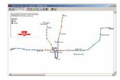
The system map module of MOWIS provides a graphical display of the entire rail system together with outstanding track defects.
