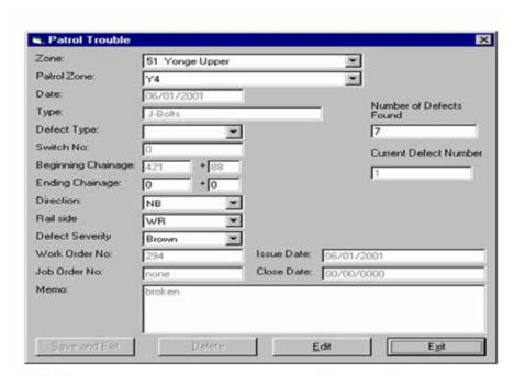
MOWIS can record and monitor track inspector defects and defect repairs.
